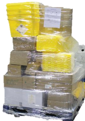
An insecurely stacked and wrapped pallet not acceptable for transit through the Palletline system
